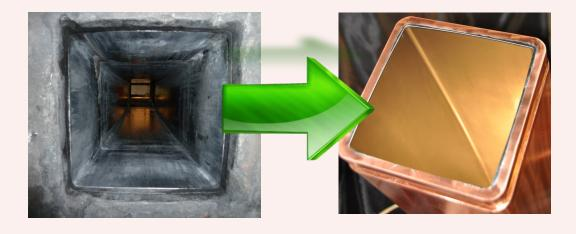
TCI refurbishes tubes sections between 130mm to 300mm and any kind of mould geometry including Single, Parabolic, Multi, Convex tapers by running 18-step-process for each tube.
